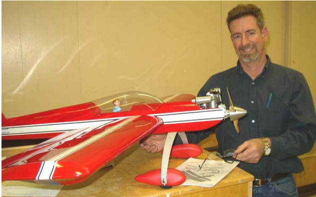
Rick Cincis shows off the Extra 300L; 49" wingspan; and is using a Saito 72 four stroke for power.
