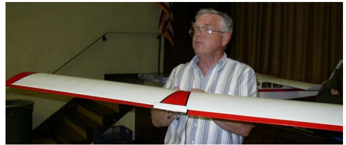
George demonstrates how a trainer wing with virtually no dihedral can pose a challenge to control but that less dihedral is better in a trainer when you are not trying to learn by yourself.
