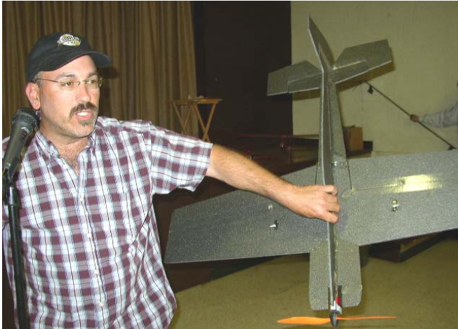
Richard tells how his foam aerobatic plane was built and of its flying characteristics. He uses a 6:1 gear drive, insulating foam and packing material hinges. The parts are not yet in kit form, but you can obtain the parts from different suppliers.
