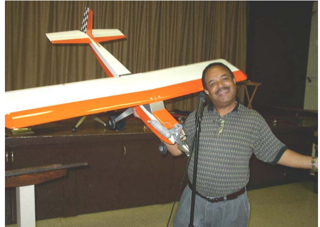
Bob used UltraCote™ on his RCM Trainer by Great Planes. ...Ta Daaa! It has a 65 inch wingspan that is fully symmetrical. Power is an MDS ABC .68 engine. Bob likes the price and how the ABC motors last.
