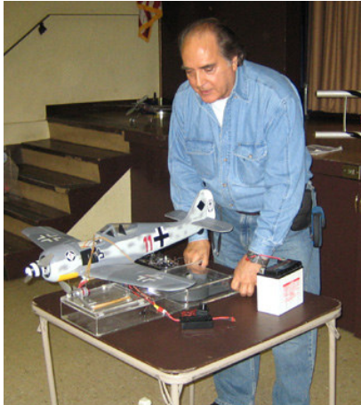
Tony DiLeo brought in a device he has made himself to measure thrust. The plane he brought in measured 12 pounds of thrust.
