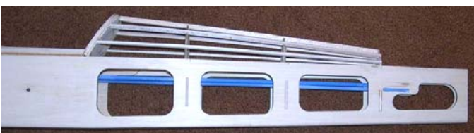
The Sullivan #505 Pushrods shown here perform much better than the generic plastic tubes included with the kit.
