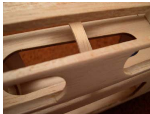
Above: Shows the optional but helpful braces I put between turtle deck stringers. Shaping them as shown was done purely for the enjoyment of the task. Right: The tail wheel section from the inside. The hard point begs for a tail wheel bracket rather than having your rudder take on landing loads via the kit's included pre-bent tail gear. Top: The nicely shaped wheel pants prior to priming.
